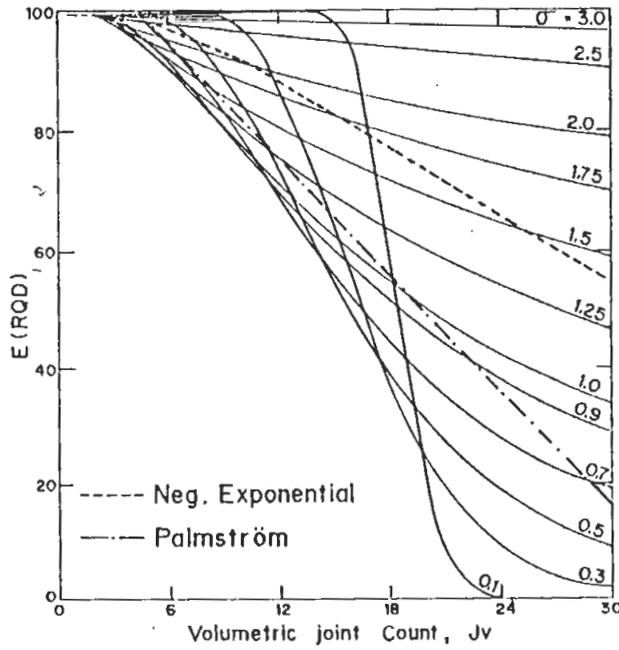
FIG. 10. Plate block  $RQD-J_v$  charts, ( $\alpha = 0.9, t = 0.10m$ ).
