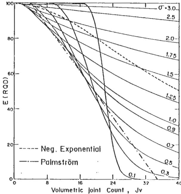
FIG. 18. Prismatic block RQD-J<sub>v</sub> charts, ( $\alpha = 0.9, \beta = 0.5, t = 0.10$  m).
