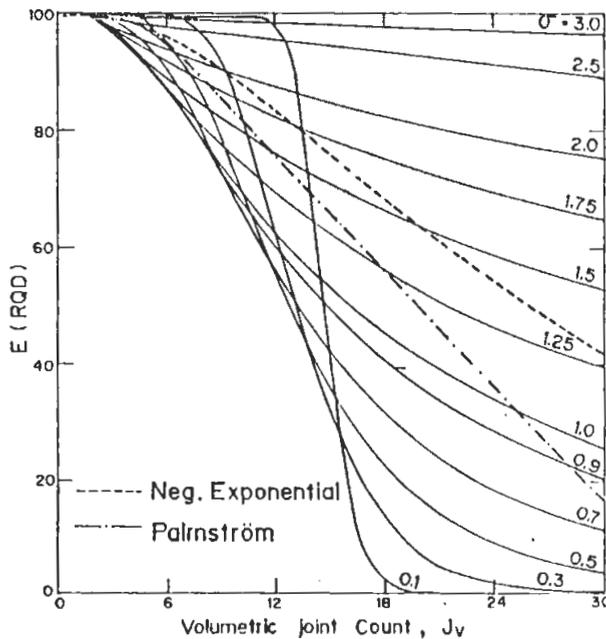
FIG. 9. Plate block *RQD*- $J_v$  charts. ( $\alpha = 0.5, t = 0.10m$ ).
