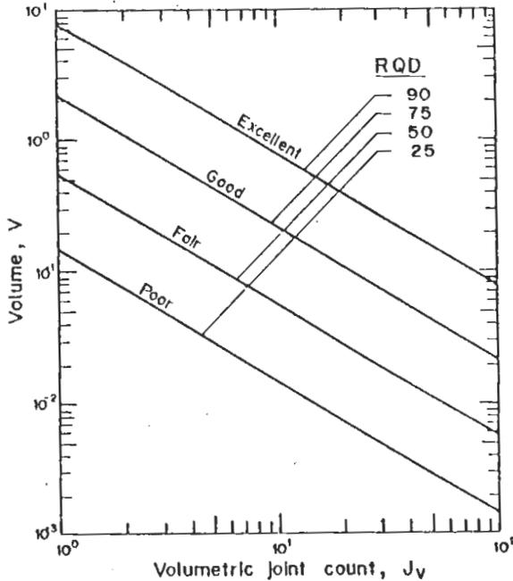
FIG. 21. Prismatic block  $RQD-J_v-V$  charts, ( $\alpha = 0.9, \beta = 0.9, t = 0.10$  m).
