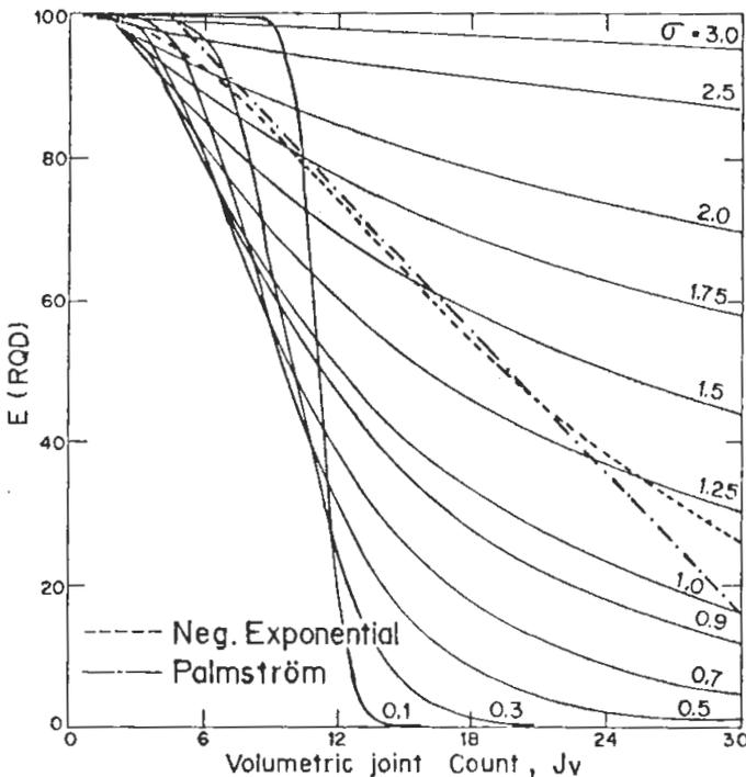
FIG. 6. Plate block  $RQD$ - $J_v$  charts, ( $\alpha = 0.1, t = 0.10m$ ).
