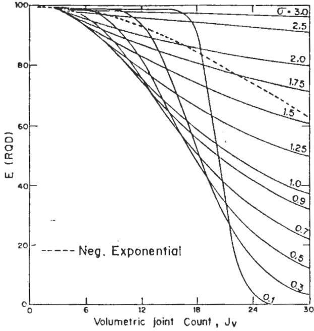
FIG. 3. Bar block  $RQD-J_v$  charts, ( $t = 0.05$  m).
