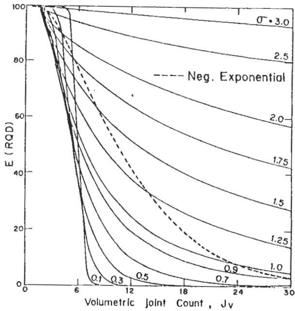
FIG. 8. Plate block  $RQD-J_v$  charts, ( $\alpha = 0.1, t = 0.20\text{m}$ ).
