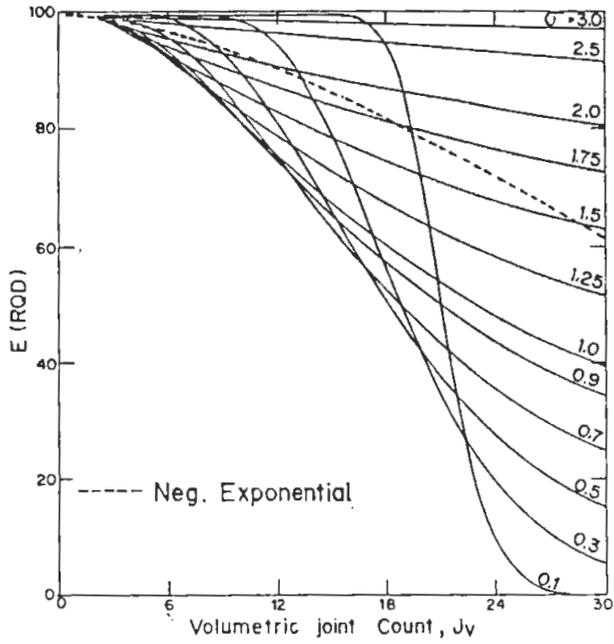
FIG. 7. Plate block  $RQD-J_v$  charts, ( $\alpha = 0.1, t = 0.05\text{m}$ ).
