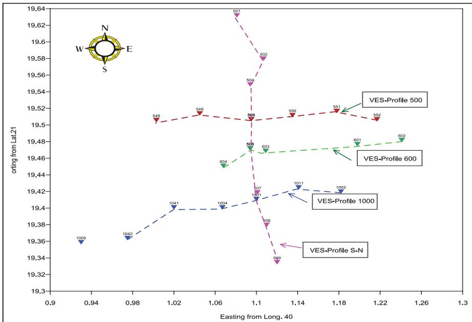
Fig. 7. Locations of vertical electrical soundings (VES).
