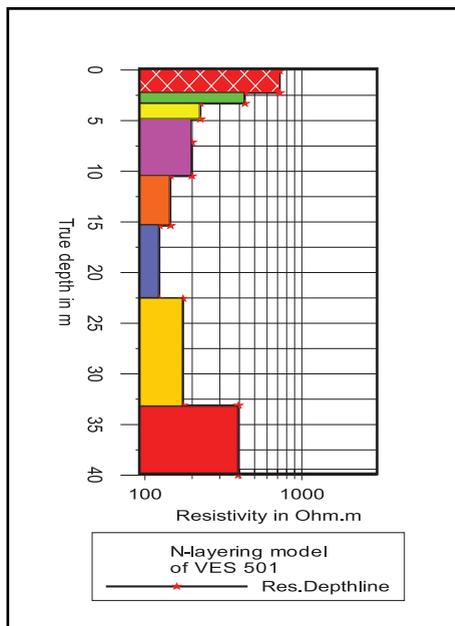
Fig. 8(b). The interpreted n-layer model.
