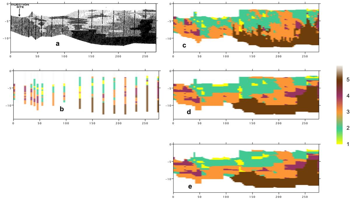
Figure 2. Comparison of different stochastic simulations of MADE1 site, shown in (a), using the calculated vertical transition probability matrix from 16 boreholes, shown in (Table 1) and assigning different horizontal transition probability matrices: (c) simulation by horizontal transition given in Table 2, (d) simulation by horizontal transition given in Table 3, (e) simulation by horizontal transition given in Table 4.
