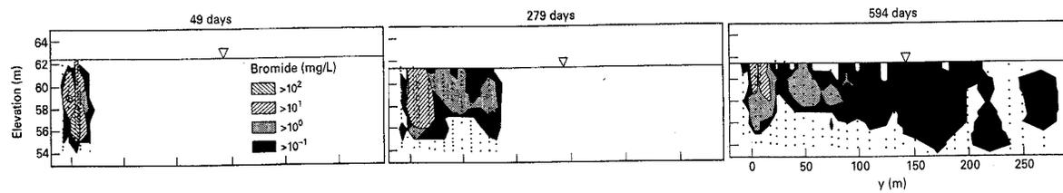
Figure 1. Three snapshots of the bromide plume at 49, 279 and 594 days [3].
