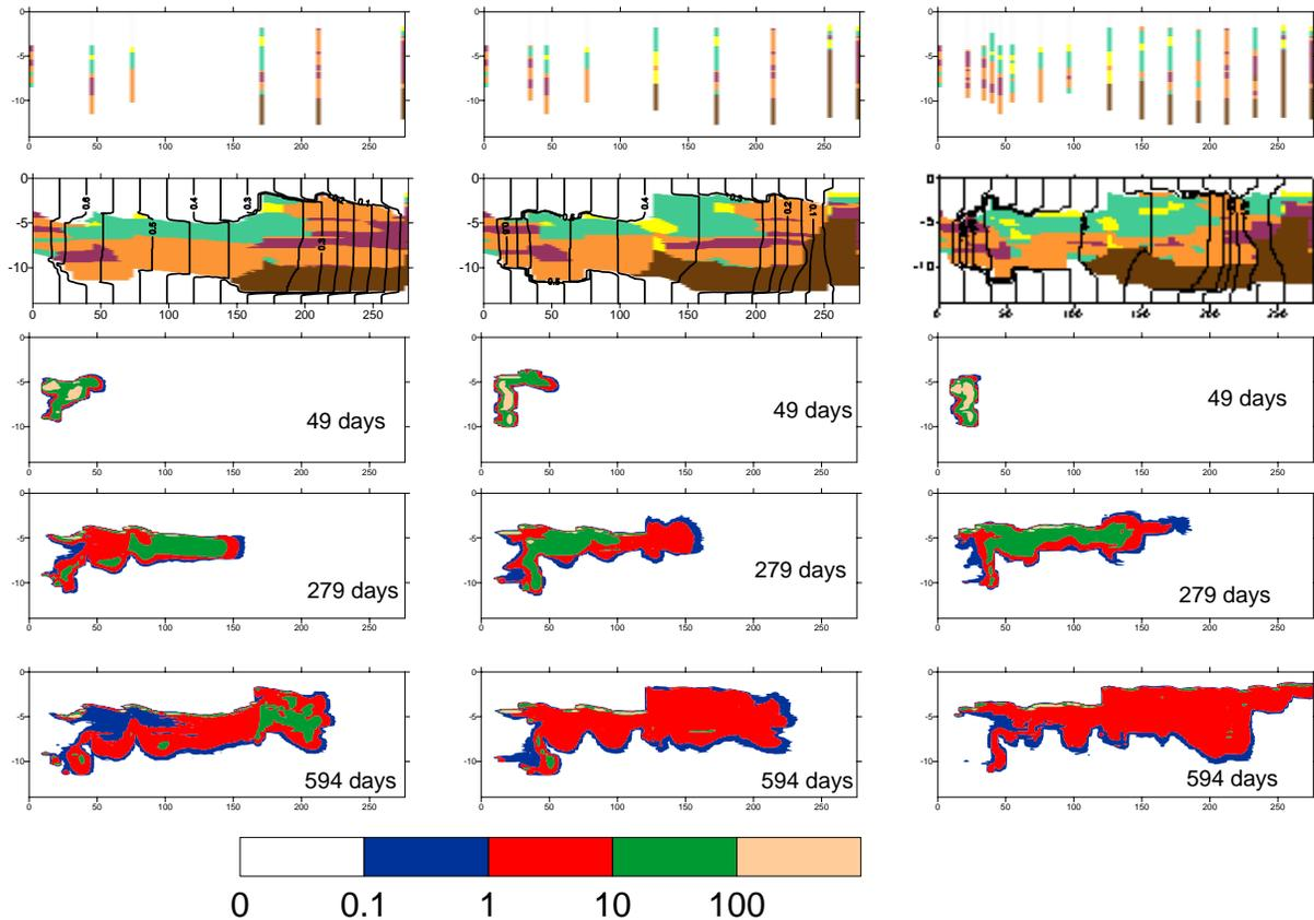
Figure 3. Comparison of numerical flow and transport simulations conditioned on number of boreholes. Left most column is a geological simulation of the aquifer conditioned on 6 boreholes with the corresponding plume evolution at 49, 279 and 594 days respectively. Second and third columns from the left side are similar to left most column but conditioned on 9 and 16 boreholes respectively. The concentration scale is in (mg/L).
